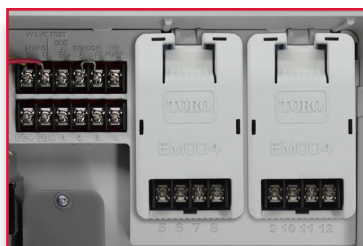
12-station configuration with (2) 4-station modules
